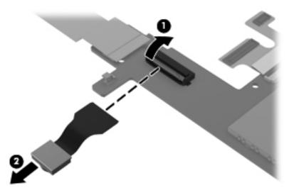
4. Remove the rear-facing webcam and cable.
